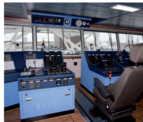
The forward facing part of the bridge, where the navigator looks out under the helipad.
