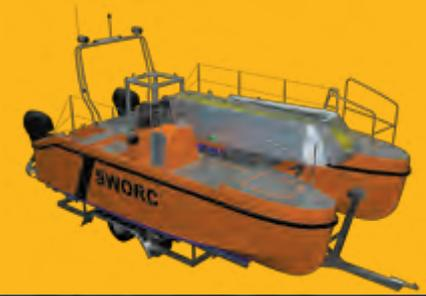
**SWORC** is designed to collect spilled oil before it reaches the shoreline, including areas of limited draft, inland and coastal waterways.
